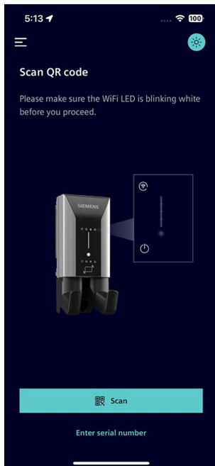
After charger has been powered on, the Wi-Fi LED should indicate that the charger is in access point mode. This can take up to five minutes. If the charger has power and the Wi-Fi LED on the charger, note what other notifications are shown on the charger display.
