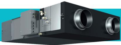
MMD-VN ventilation products are using exhaust air + DX-coil to pre-condition the incoming air, thus reducing the cooling load and the overall size of the required air conditioning system.
