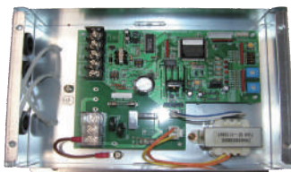
Modbus® Interface TCB-IFMB641TLE
